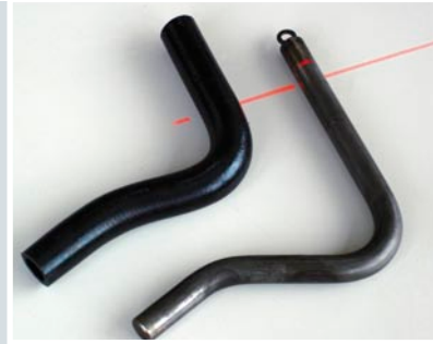
Hose-mandrel comparison – graphic generation of scan data and simultaneous data output in 3D and bending format including data correction according to bender model
